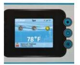
Press ((Top left) jet button to activate some of the hydromassage jets, you will see the jet 1 icon on the screen rotate.
