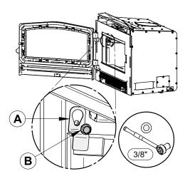
Figure 14: Install the Combustion Chamber Bricks
