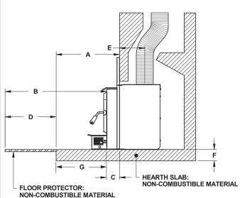
Figure 10: Additional Floor Protection - Not Raised Installation
