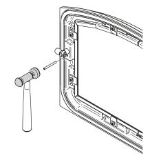
Figure 12: Installing the split pin
