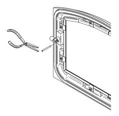
Figure 11: Removing the split pin
