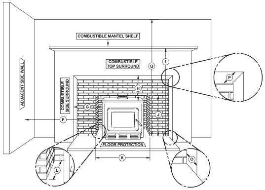
Figure 7: Hearth opening and clearances to combustibles
