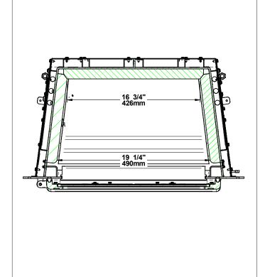
Figure 5: Top View - Combustion Chamber
