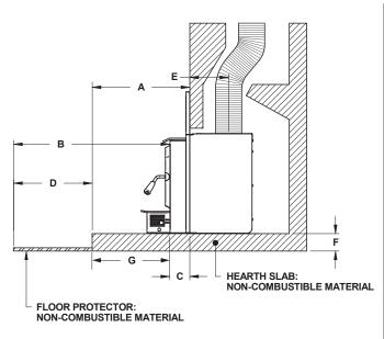
Figure 9: Additional Floor Protection - Raised Installation
