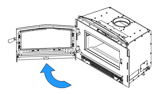
2. Hold the fire screen by the two handles and bring it close to the door opening.
