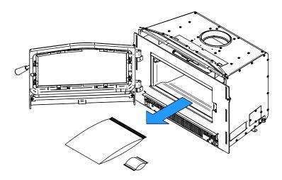
Figure 13: Empty the combustion chamber
