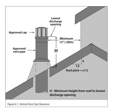
Minimum height (H) from roof **Roof Pitch** Feet Meters Flat to 6/12 0.30 1.0 Over 6/12 to 7/12 1.25 0.38 Over 7/12 to 8/12 1.5 0.46 Over 8/12 to 9/12 2.0 0.61 Over 9/12 to 10/12 2.5 0.76 Over 10/12 to 11/12 3.25 0.99 Over 11/12 to 12/12 4.0 1.22 Over 12/12 to 14/12 5.0 1.52 Over 14/12 to 16/12 6.0 1.83 Over 16/12 to 18/12 7.0 2.13 Over 18/12 to 20/12 7.5 2.27 Over 20/12 to 21/12 8.0 2.44
