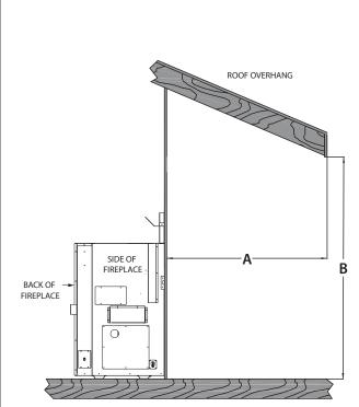
The overhang (A) must be a minimum of 1/2 or greater of the roofline elevation (B) above the base of the fireplace.
