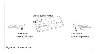
IMPORTANT: Slight adjustments to the venturi opening will create dramatic results. Adjust at slight increments until desired look is achieved. Always burn the fireplace for at least 15 minutes, and allow the appliance ample time to cool before making any further adjustments.
