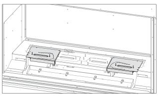
Figure 8.13, Control Board Removal and Installation - 1
