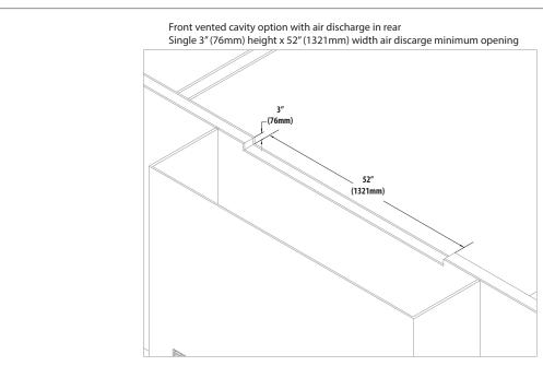
Figure 3.17, Vented Cavity Rear to Adjacent Room Installation
