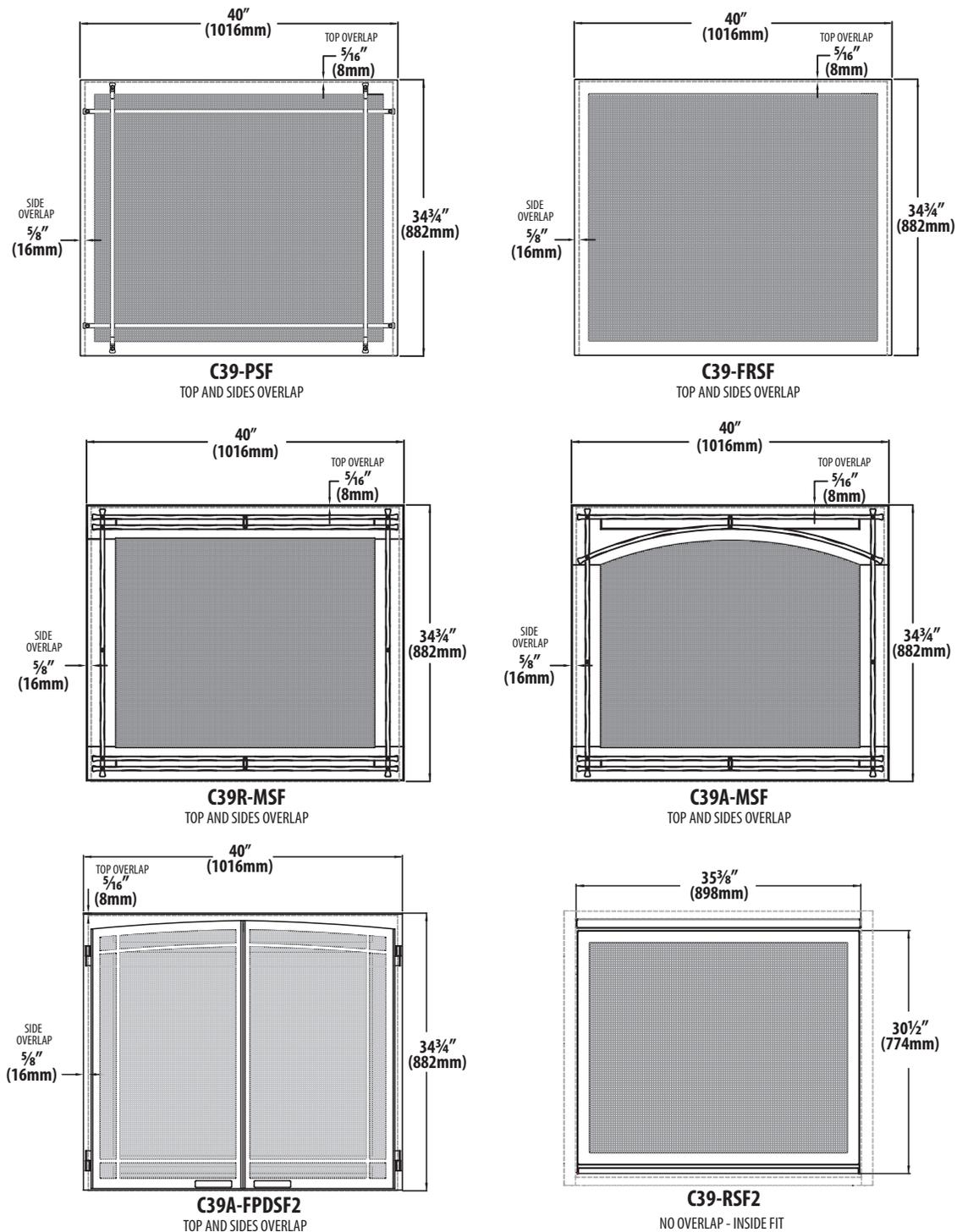
FIGURE 2.2 Safety Barrier Dimensions
