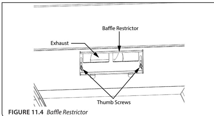
FIGURE 11.4 Baffle Restrictor
