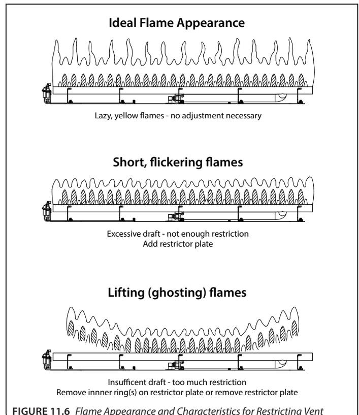
FIGURE 11.6 Flame Appearance and Characteristics for Restricting Vent
