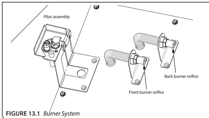
FIGURE 13.1 Burner System
