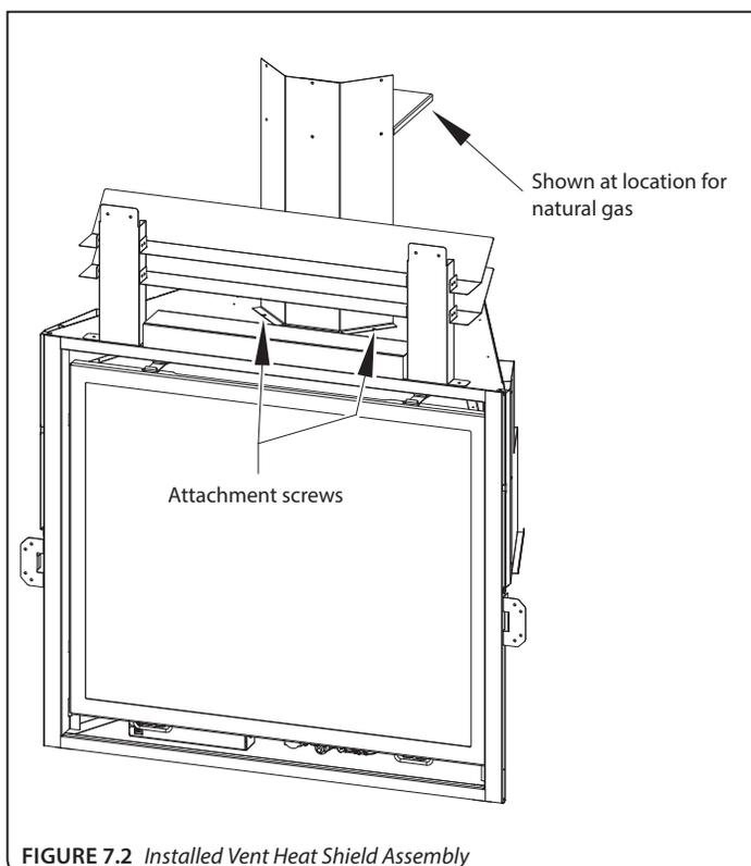
**FIGURE 7.2** Installed Vent Heat Shield Assembly
