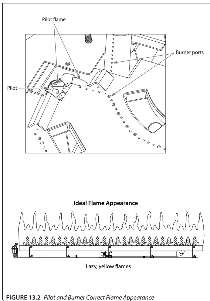
FIGURE 13.2 Pilot and Burner Correct Flame Appearance
