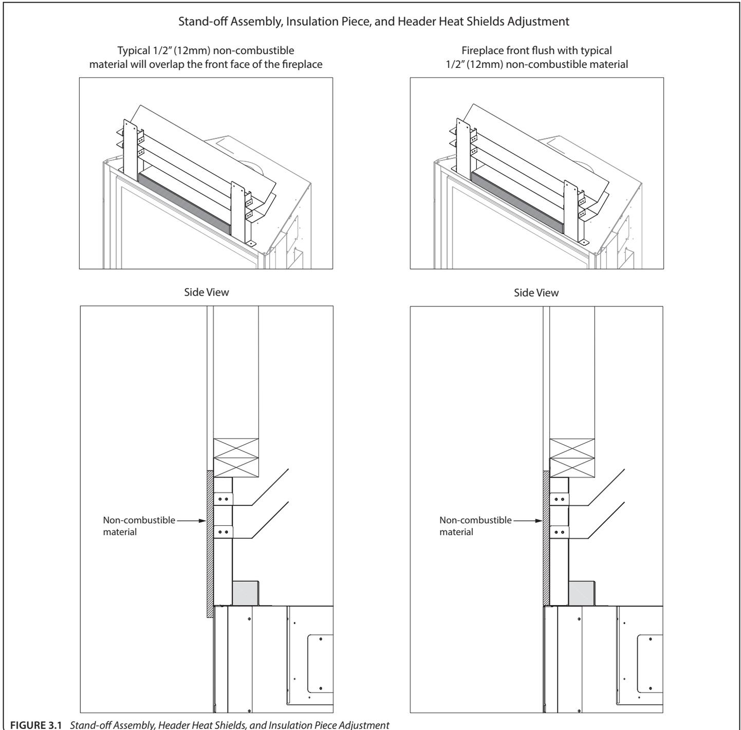
FIGURE 3.1 Stand-off Assembly, Header Heat Shields, and Insulation Piece Adjustment
