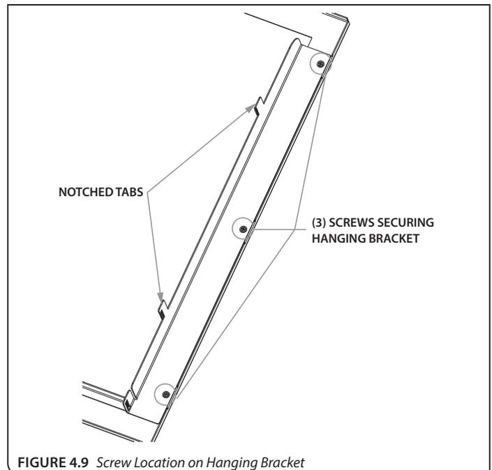
FIGURE 4.9 Screw Location on Hanging Bracket
