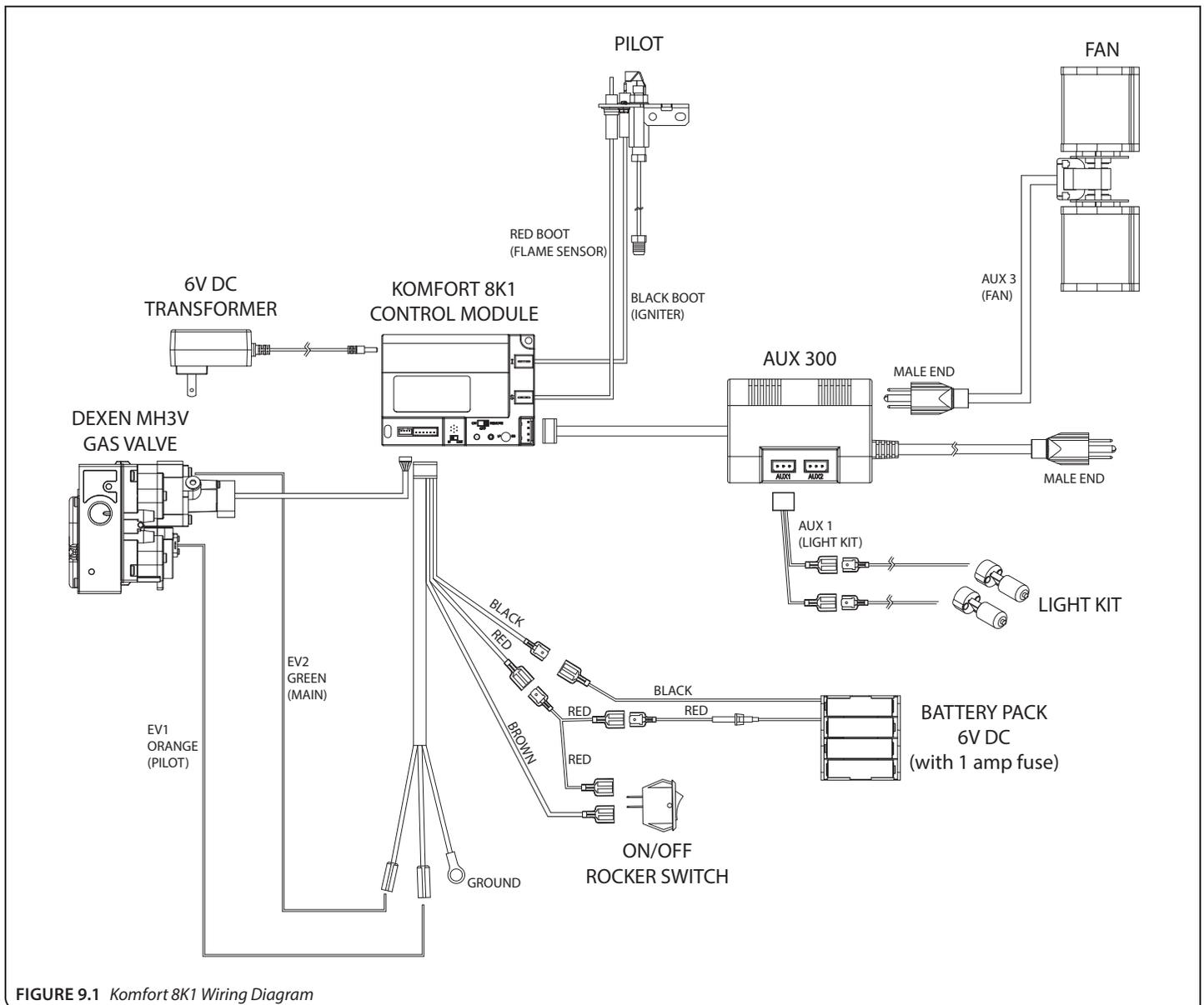
FIGURE 9.1 Komfort 8K1 Wiring Diagram
