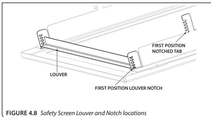
FIGURE 4.8 Safety Screen Louver and Notch Locations
