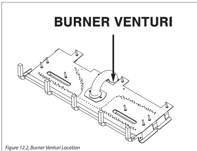
**IMPORTANT:** Slight adjustments to the venturi opening will create dramatic results. Adjust at slight increments until desired look is achieved. Always burn the fireplace for at least 15 minutes, and allow the appliance ample time to cool before making any further adjustments.
