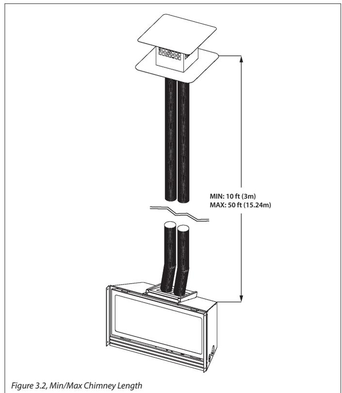
Figure 3.2, Min/Max Chimney Length
