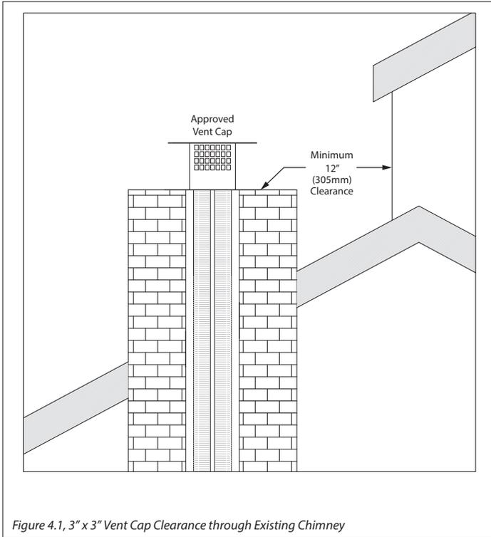
Figure 4.1, 3" x 3" Vent Cap Clearance through Existing Chimney
