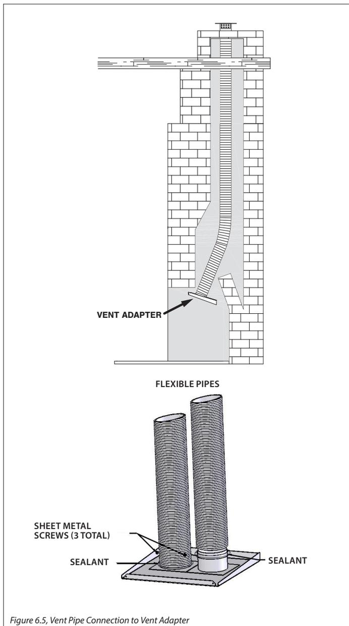
Figure 6.5, Vent Pipe Connection to Vent Adapter
