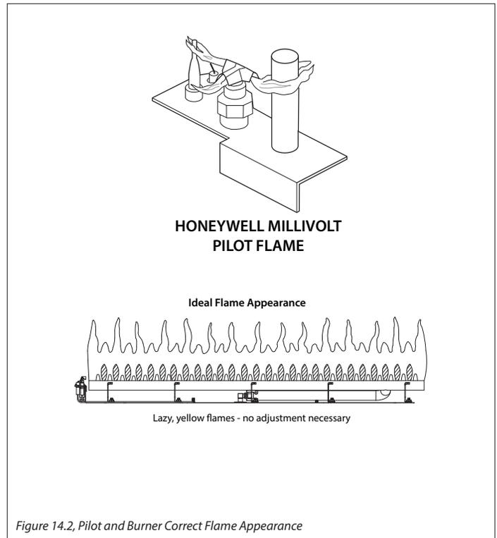
Figure 14.2, Pilot and Burner Correct Flame Appearance
