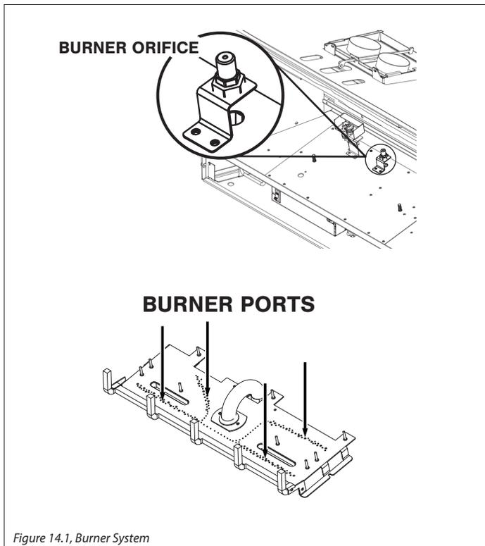
Figure 14.1, Burner System
