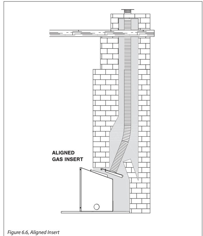
Figure 6.6, Aligned Insert
